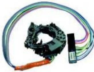
CLAVE: S36616 NUM. PARTE: SW776 SWITCH DE DIRECC AUTOMOTIVE BUICK ESTATE WAGON 94-96; REGAL SEDAN / COUPE 94-96; CHEVROLET LUMINA 95-01; MONTE CARLO 95- 99; CUTLASS / CUTLASS SUPREME 95-97; PONTIAC GRAND PRIX 94-96. 19005031, 1995955, D6226A TW49 36A061 TW 12 HILOS
