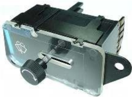
CLAVE: S39133 NUM. PARTE: WS-1003 SWITCH DE LIMPIADORES AUTOMOTIVE GM TRUCKS 78-83 39G13 47A010
