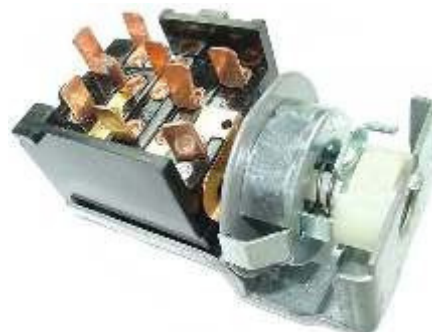
CLAVE: S10805 NUM. PARTE: HS-108-K1 SWITCH DE LUZ AUTOMOTIVE P/DODGE "K" 1 TERMINAL CHRYSLER CORDOBA 75-83; DYNASTY 88-93; IMPERIAL 75, 81-83, 90-93; LEBARON 77-83, 89, 91-93; NEW YORKER 75-86, 88-92; TOWN & COUNTRY 75-87; DODGE CHARGER 73-78, 83-87; MAGNUM 78-79; MONACO 75-78; NEON 95-96; SHADOW 87-94; SPIRIT 89-92; VIPER 92-96; DODGE LIGHT TRUCK CARAVAN 7 GRAND CARAVAN 84-87; DAKOTA 87-96; PICK UP FULLSIZE / RAM CHARGER 79-93; VAN FULLSIZE 78-87; VAN MINI RAM 84-87; JEEP CHEROKEE 92-93; GRAND CHEROKEE 93; PLYMOUTH NEON 95-96 VOYAGER / GRAND VOYAGER 84-87. DS-357 HL-6548 39A005-B
