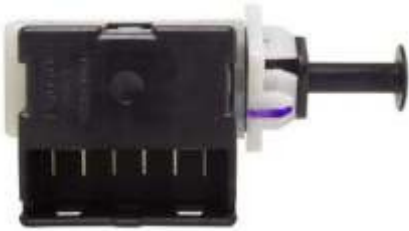
CLAVE: S24080 NUM. PARTE: SW5437 SWITCH DE STOP AUTOMOTIVE CHRYSLER SEBRING (09-10), DODGE AVENGER, CALIBER, JOURNEY (09-10), JEEP COMMANDER (06-10), JEEP COMPASS, PATRIOT (09-10), JEEP GRAND CHEROKEE (05-10) 48A042 56054001AB ARTICULO NUEVO
