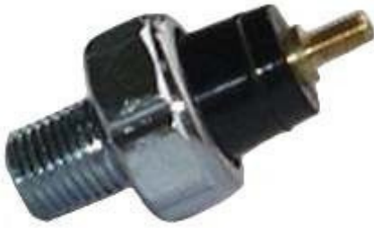
CLAVE: B15108 NUM. PARTE: OP-6615 BULBO DE ACEITE AUTOMOTIVE FORD 67-72, 74-77, 96-99, TRUCK 67-74, LINCOLN 68-69, 72-77, MERCURY 69-72, 75-77 1/4" x 18, 3.0-8.3 PSI. PS57 28A001 15G10
